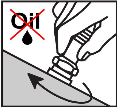
USE A TORQUE WRENCH FOR INSTALLATION OF SPARK PLUGS
